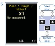
Use the Arrow buttons to switch between the points in route
