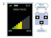
Adjust the brightness with the Arrow buttons
