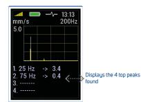
FFT analysis of vibrations: 1 - 200 Hz in mm/s (ips) RMS
