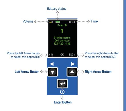
To open the Basic menu press the Enter button (on any measurement screen)
