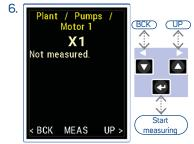
[BCK] go back to point selection [UP] go back to machine selection Press the Enter button [MEAS] to start measuring
