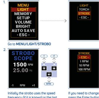
frequency (if it is known) or the last speed from memory. The step (1, 10, 100 RPM) is displayed on the bottom line of the screen.
